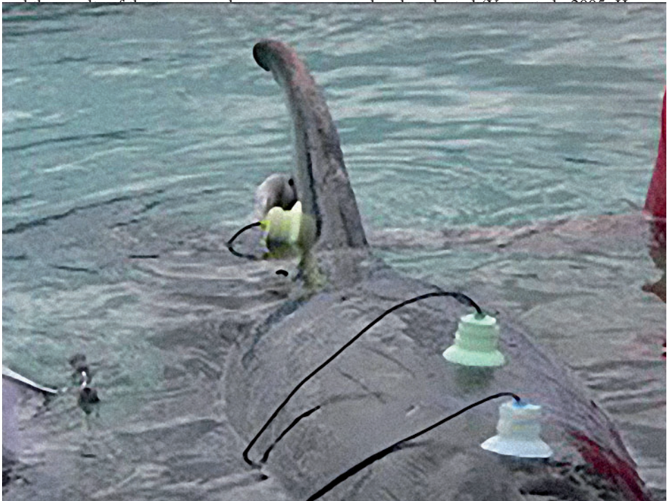
Fig. 1: Suction cups containing surface electrodes attached to a beached cetacean. Photo: Marine Mammal Research Program, University of Hawaii
