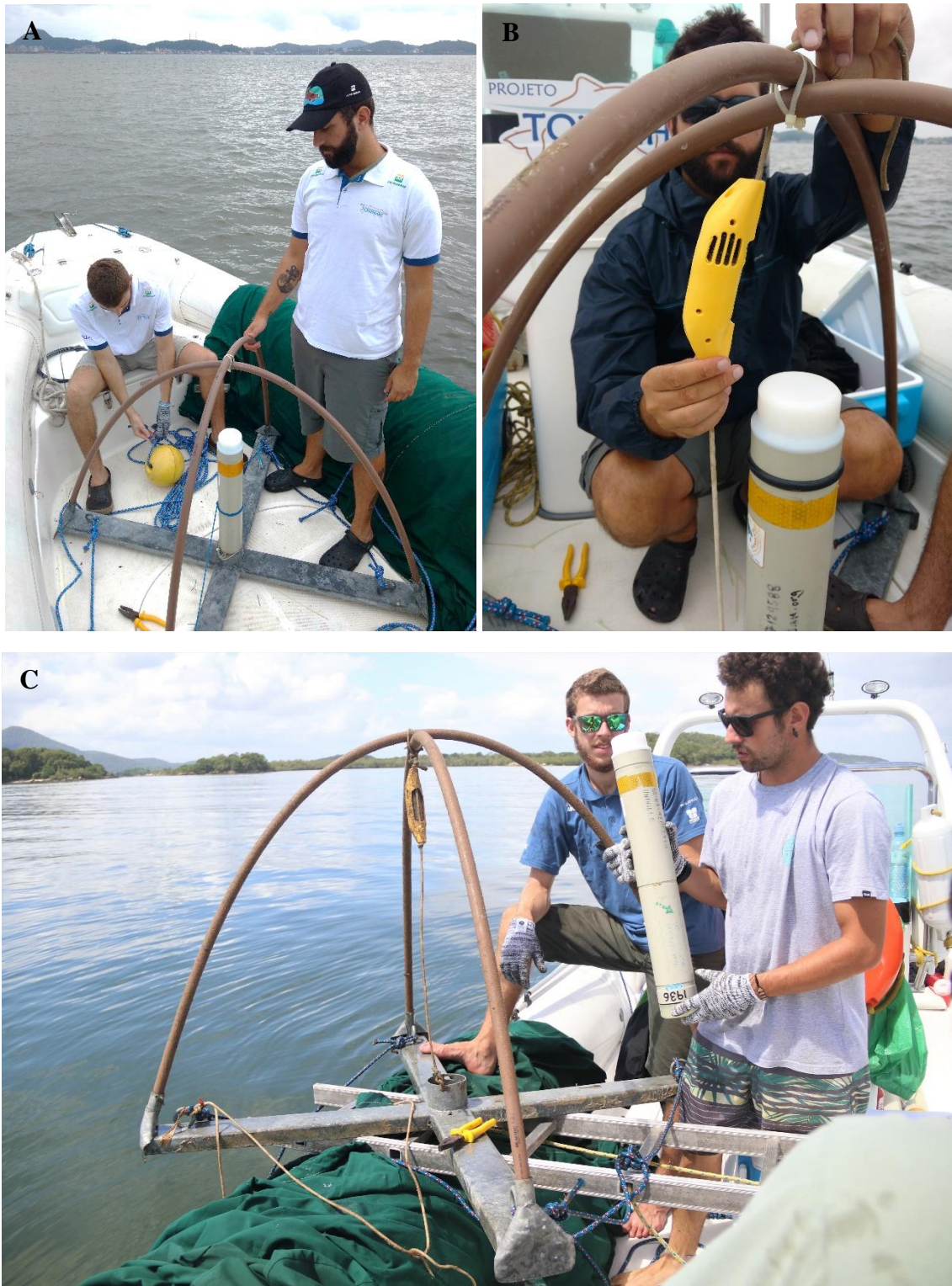
Figure 3: Toninhas Project team performing the installation of a Static Acoustic Monitoring equipment (C-PODs - Chelonia Limited) in Babitonga Bay (A) and an acoustic repellent (Banana Pinger - Fishtek Marine) (B). One can observe the cages that were specially designed for protection and anchorage of the acoustic equipments (C).
